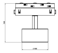
Dimensions: Φ100 x 148mm Total power: 12 w Luminaire luminous flux: 1200 lm Luminaire efficacy: 100 lm/w Weight: 2 kg
